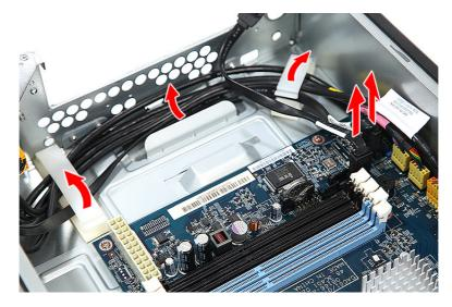
5. Disconnect the front I/O board and card reader board cables from their mainboard connectors.
